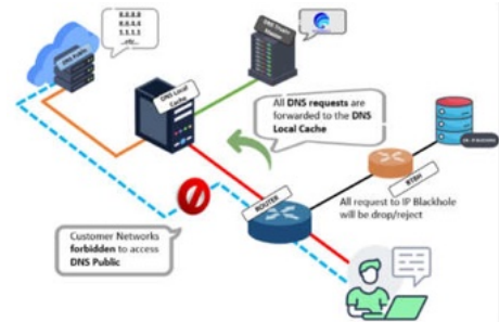
Figure 1. Design of the DNS Trust+ and RTBH System in Wareng Village [4]
